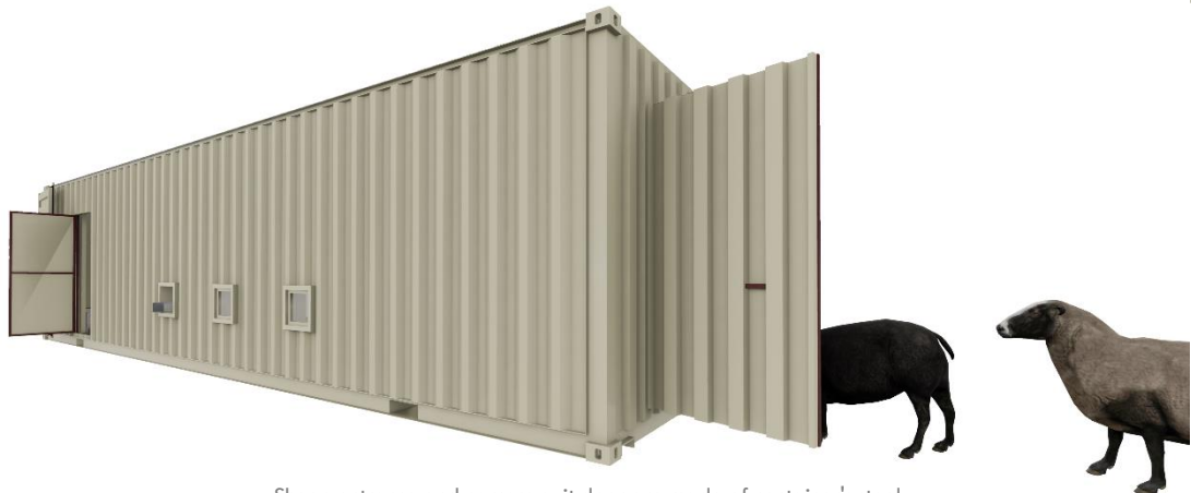
Sheep entrance and carcass exit door are made of container's steel. Container sheet will be cut and turned into a hinged door.
